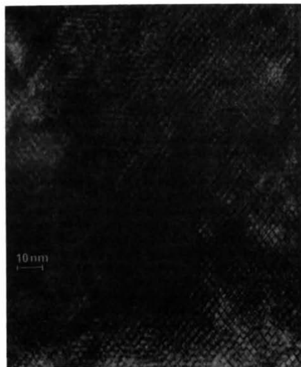
Fig. 6. A (110) high-resolution image of an NaCl-type region showing the general aspect of this structure. A mesh of lozenge-shaped domains is clearly visible.
